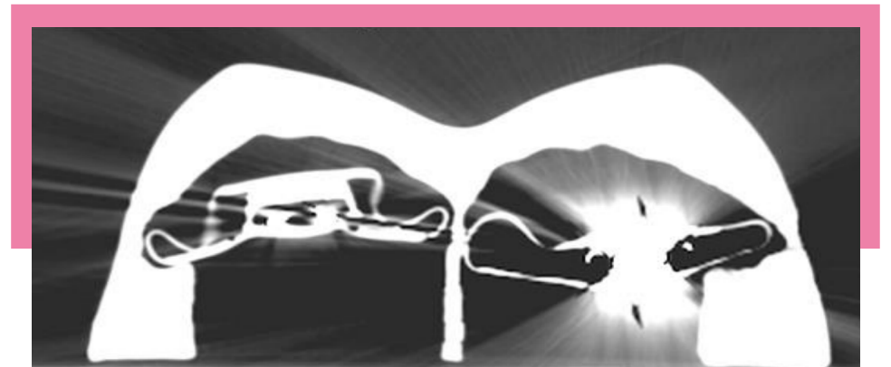
Comparison of artifacts in a CT scan of a phantom with (left) Motiva Flora® Tissue Expander and (right) a tissue expander with ferromagnetic components.
